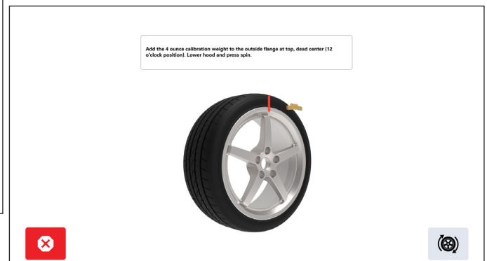
Figure 53- Apply 4 Oz. Calibration Weight to Outboard Clip Flange
