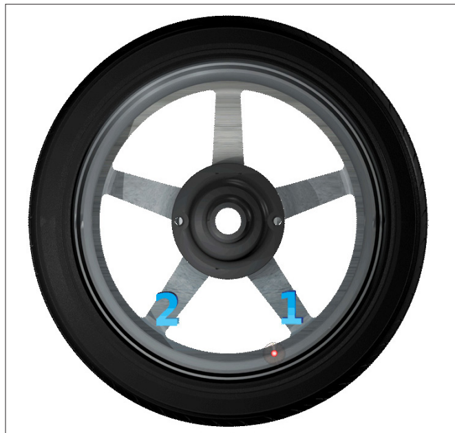
Figure 40 - Spoke 1 and Spoke 2 Locations on Either Side of Original Outboard Weight Location
