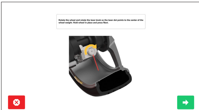
Figure 55 -- Align Laser Dot With the Center of the Cal Weight
