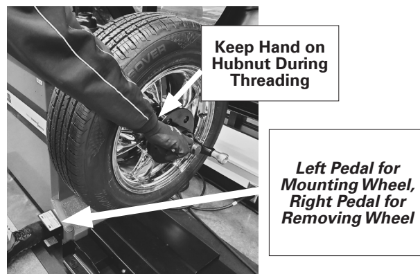
Figure 61 - Mounting Wheel Assembly Using Foot Pedal Threading
